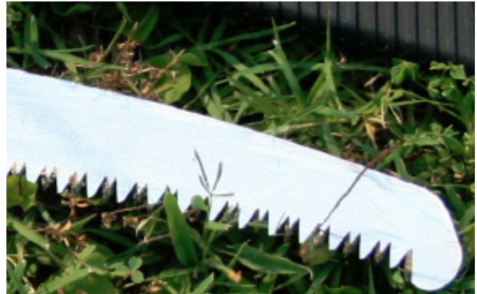
Figure 2.4. Two types of turbo handsaws (top)—both cut on the pull stroke. Close-up of a tri-cut or turbo blade (bottom).
