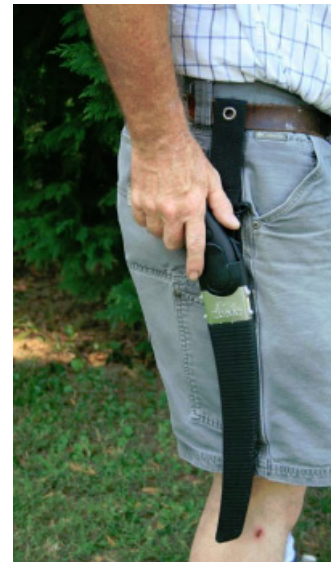
Figure 2.5. Most scabbards have a loop that allows you to attach a saw to your belt or a climbing saddle.
